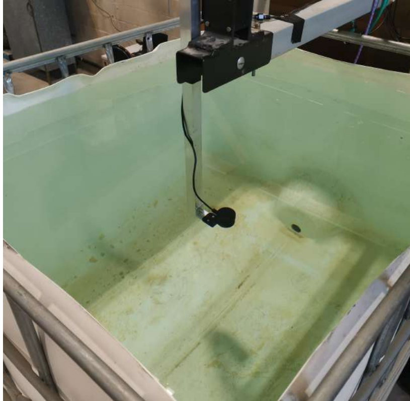
Figure 4.2: Experimental setup for collecting profile data at different distances with the sensor facing upwards towards the PAR surface.
