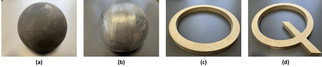
Figure 3.1: The different types of targets used for the experiments. (a) is the whole polyurethane sphere, (b) is the hollow aluminum sphere, (c) is the MDF O and (d) is the MDF Q. Images taken from Blanford et al. (2024)
