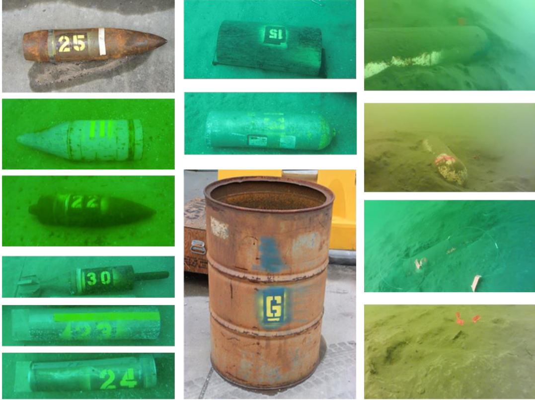
Figure 2.2: Selection of targets deployed during TREX13. (left) Munitions targets, including bullet-shaped and finned UXO, a TP-T round, and an aluminum cylinder/pipe. (middle) Clutter items, including a telephone pole section, a scuba tank, and a 55-gallon drum. (right) Illustration of target burial state on the seafloor[31].
